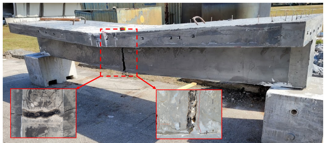
Figure 6. Failure mode of the retrofitted T-beam, illustrating strain localization in the web.
