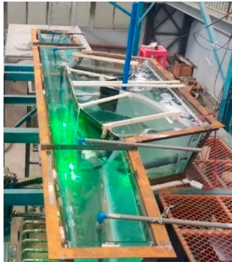
**Figure 3.** On-site pictures of the six-strand tundish water model.
