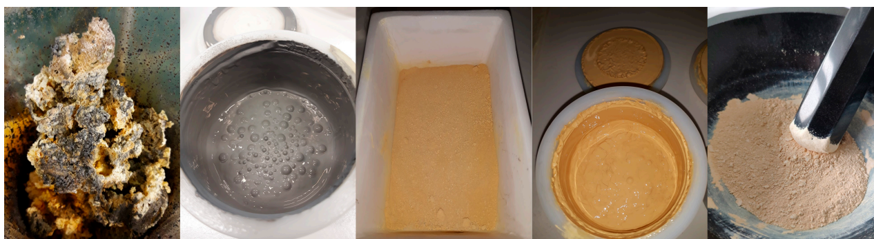
Figure 3. Illustration of the preparation of the 9/65/35 PLZT:Pr 3+ powder, obtained via gel-combustion synthesis and calcined at T = 600^\circ\text{C}/4 h.
