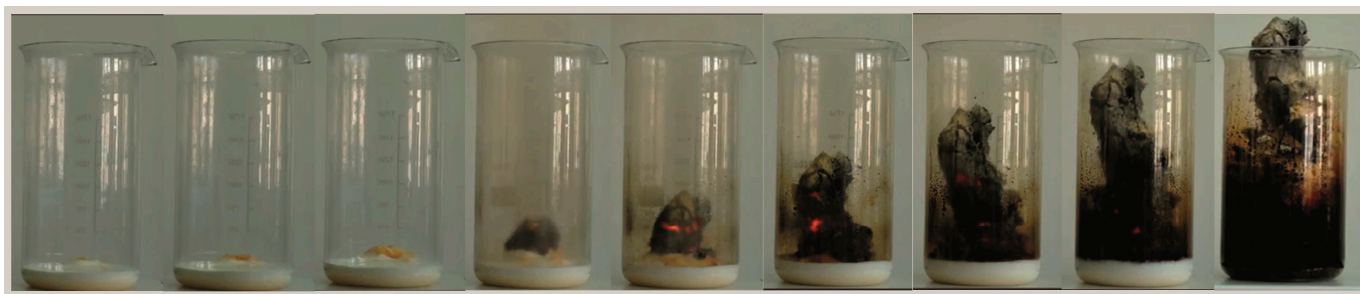
Figure 2. An example of the low-temperature synthesis of 9/65/35 PLZT:Pr 3+ powders by gel-combustion method.
