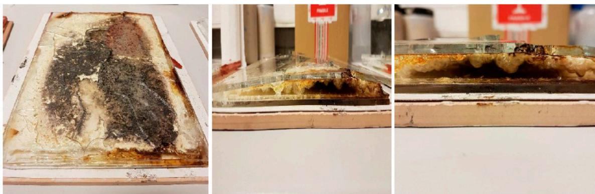
**Figure 7.** Exemplary glass mold with a hydrogel filling after the fire test (sample 5%/1:9 (20 wt.% of ANa aq.)).
