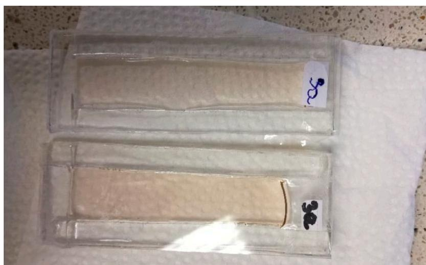
**Figure 10.** Exemplary hydrogel samples prepared for the transluency measurement (sample 5%/1:9 with 20 wt.% ANa aq.: upper sample—no aging, 2 mm of gel, bottom sample—no aging, 4 mm of gel).
