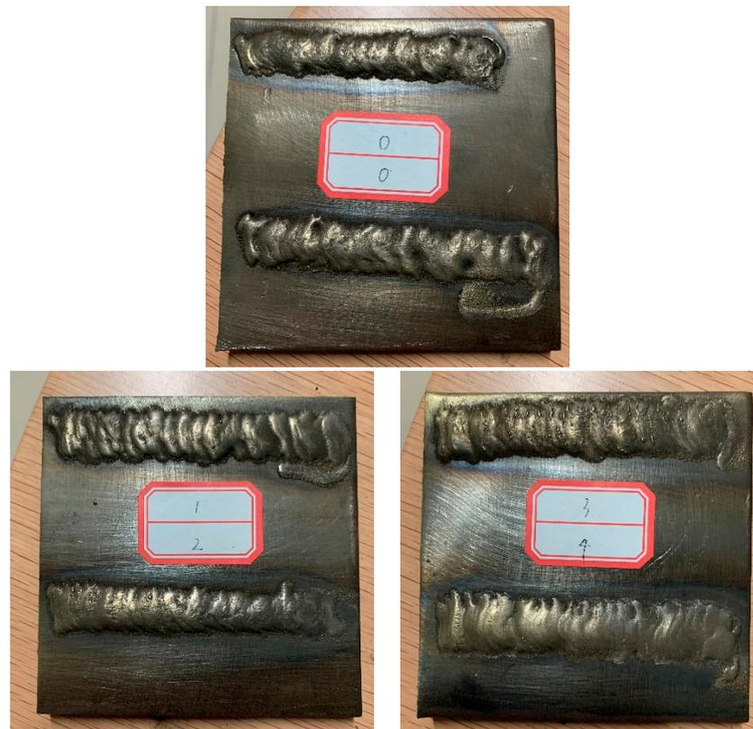
**Figure 3.** Picture of HEA and XZrC coatings: (0) HEA; (1) 01ZrC; (2) 02ZrC; (3) 03ZrC; (4) 04ZrC.
