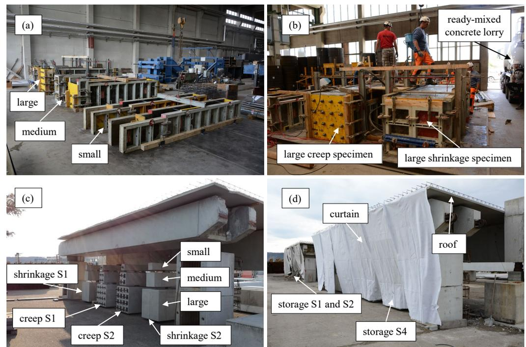
**Figure 3.** Production and storage of the large-scale specimens. (a) Formwork for the specimens of series S1. (b) Casting of the large specimens of series S1. (c) Storage of the specimens of series S1 and S2 before installation of the curtain. (d) Final storage of the test series.
