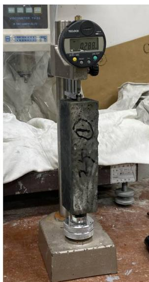
Figure 8. Testing drying shrinkage.
