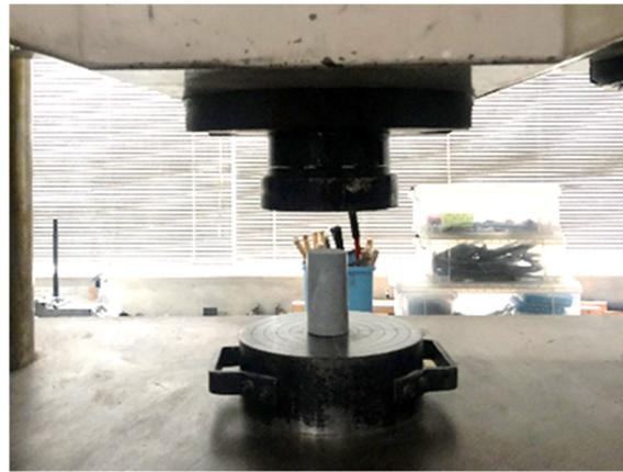
Figure 5. The testing of compressive strength (200 kN capacity).
