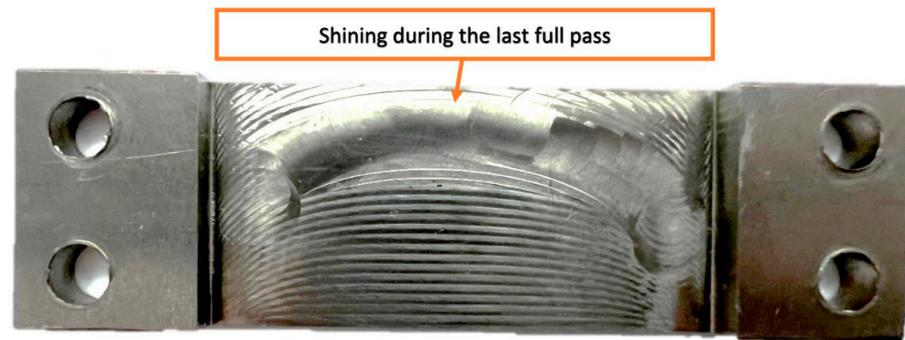
**Figure 9.** Shining of the machined surface of a sample with a horizontal thin wall appearing during the last full pass.
