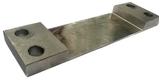
**Figure 4.** Representation of a sample with a thin wall in horizontal orientation.
