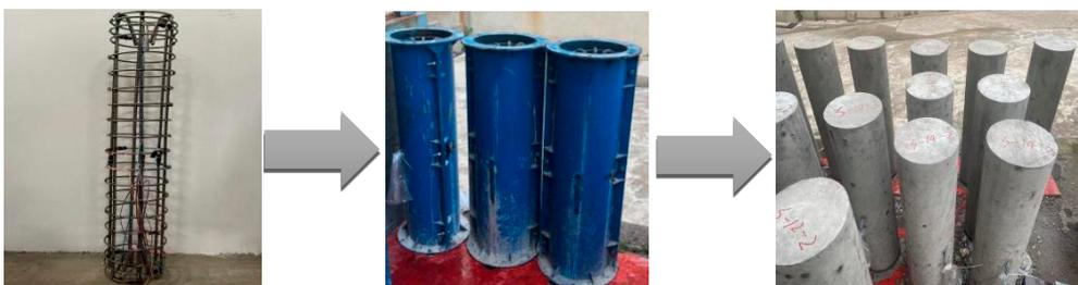
**Figure 3.** Preparation process of short columns.
