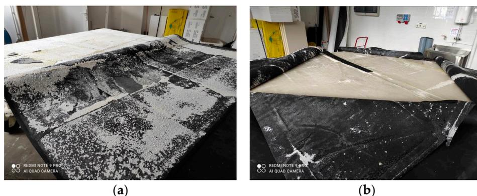
**Figure 5.** Nature of the roof covering pulling off. (a) EPDM laminated to EPS substrate, (b) EPDM with no lamination from the EPS substrate.
