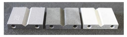
**Figure 5.** From left to right, a consolidated aluminum metal part as-printed, smut-treated, and a desmutted sample.
