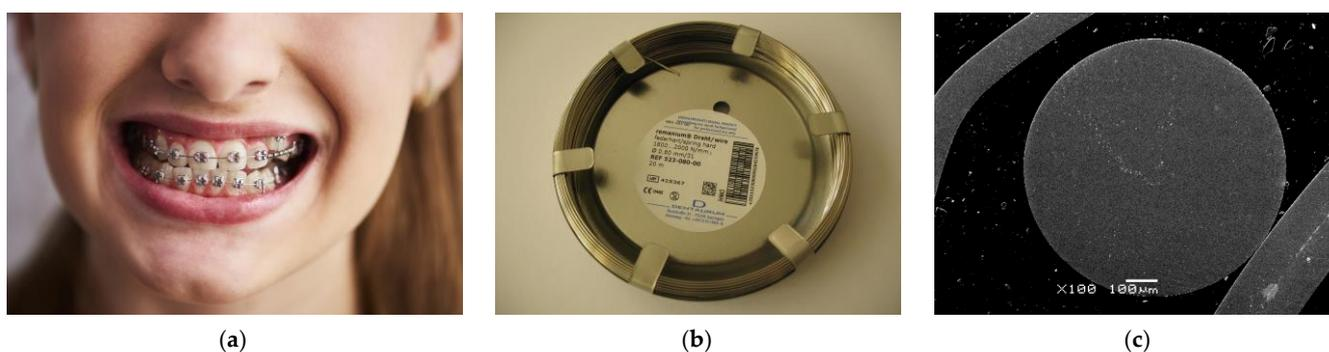
**Figure 1.** Dentaurum Remanium® archwire: (a) in the orthodontic apparatus as arches [22]; (b) in trading condition; (c) SEM image of the sample after inclusion in graphite.
