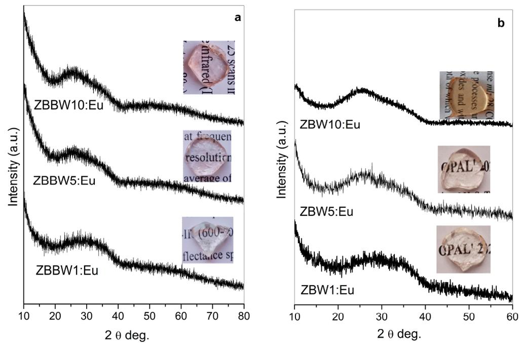
**Figure 1.** XRD patterns of (a)  $50\text{ZnO}:(49-x)\text{B}_2\text{O}_3:1\text{Bi}_2\text{O}_3:x\text{WO}_3:0.5\text{Eu}_2\text{O}_3$ ,  $x = 1, 5$ , and  $10$  mol%; (b)  $50\text{ZnO}:(50-x)\text{B}_2\text{O}_3:x\text{WO}_3:0.5\text{Eu}_2\text{O}_3$ ,  $x = 1, 5$ , and  $10$  mol%.
