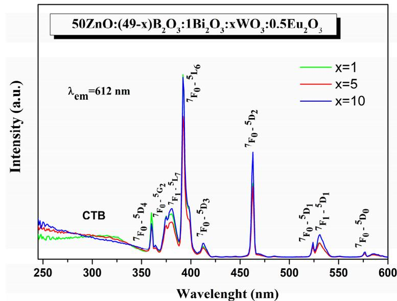
Figure 6. Excitation spectra of  $50\text{ZnO}:(49-x)\text{B}_2\text{O}_3:1\text{Bi}_2\text{O}_3:x\text{WO}_3:0.5\text{Eu}_2\text{O}_3$  ( $x = 1, 5,$  and  $10$  mol%) glasses.
