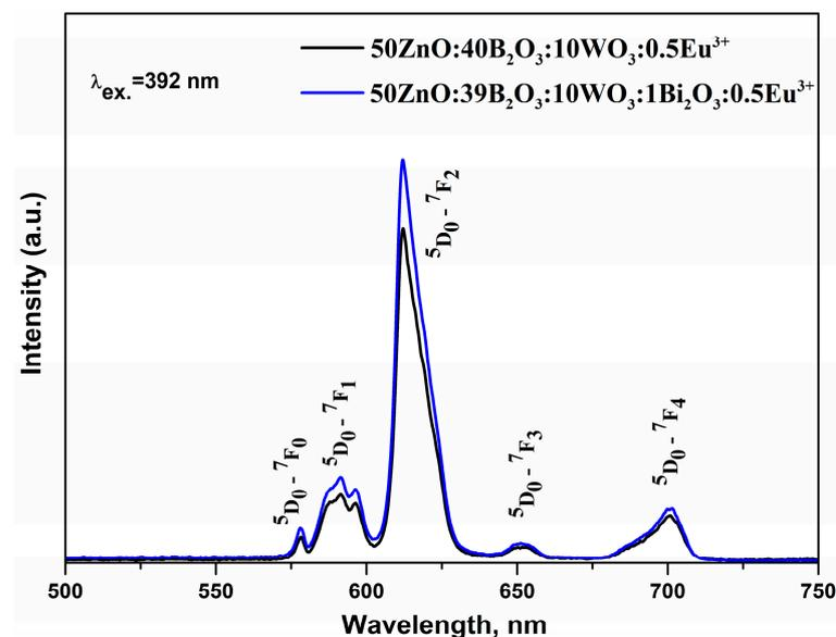
**Figure 8.** Emission spectra of  $50\text{ZnO}:(40 - x)\text{B}_2\text{O}_3: x\text{Bi}_2\text{O}_3:10\text{WO}_3:0.5\text{Eu}_2\text{O}_3$  ( $x = 0$  and  $1$  mol%).
