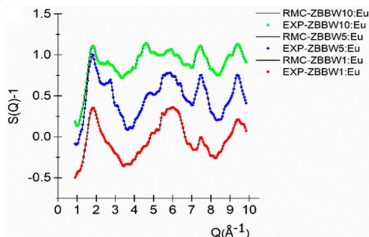
**Figure 4.** Experimental (color) and RMC (black line)-simulated neutron scattering structure factors for  $50\text{ZnO}:(49-x)\text{B}_2\text{O}_3:1\text{Bi}_2\text{O}_3:x\text{WO}_3:0.5\text{Eu}_2\text{O}_3$ ,  $x = 1, 5$ , and  $10$  mol% glasses.
