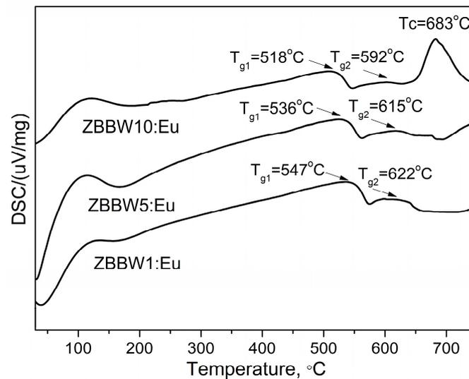
**Figure 2.** DSC curves of glasses  $50\text{ZnO}:(49-x)\text{B}_2\text{O}_3:1\text{Bi}_2\text{O}_3:x\text{WO}_3:0.5\text{Eu}_2\text{O}_3$ ,  $x = 1, 5$ , and  $10$  mol%.
