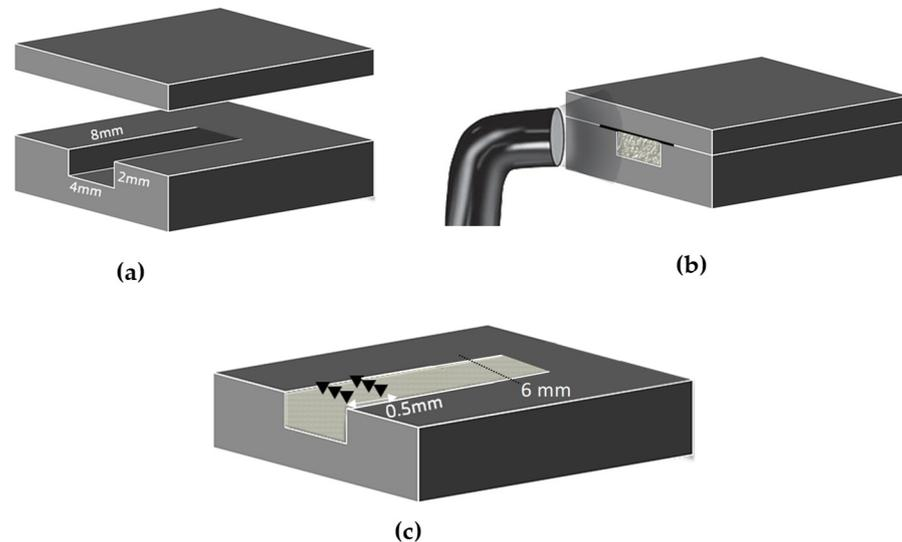
**Figure 1.** The stainless steel mold for the depth of cure specimens' preparation. (a) The mold's dimensions and the cover plate; (b) the tested material was placed and secured with the cover plate and Mylar strip in between (black line); and then a light-cured (c) illustration of the indentations (black triangles) for the Vickers hardness test.
