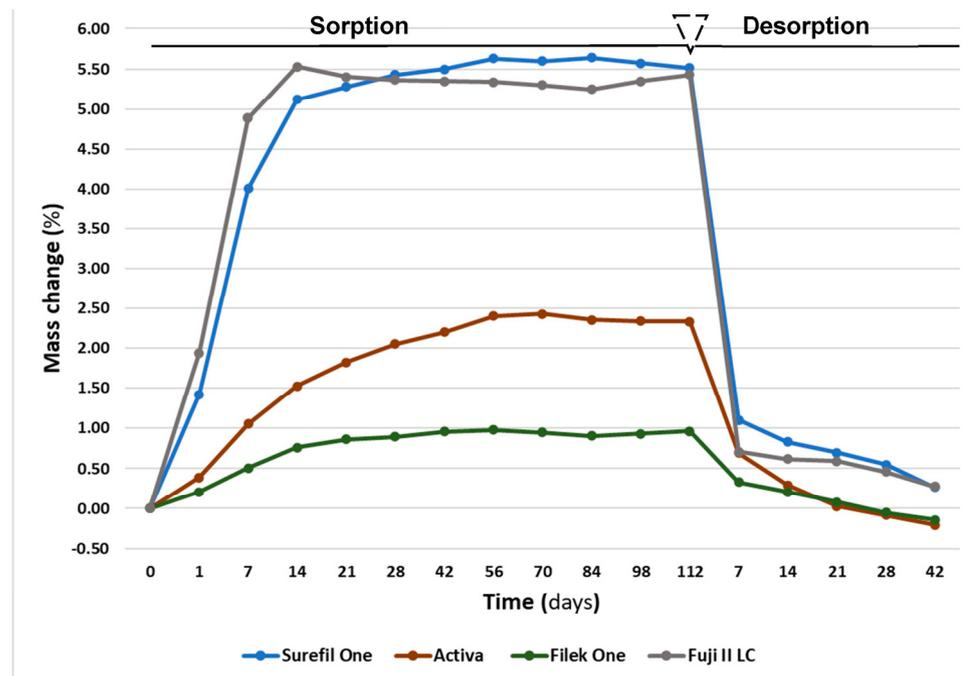
**Figure 3.** Mass change percentage with water sorption and desorption cycles.
