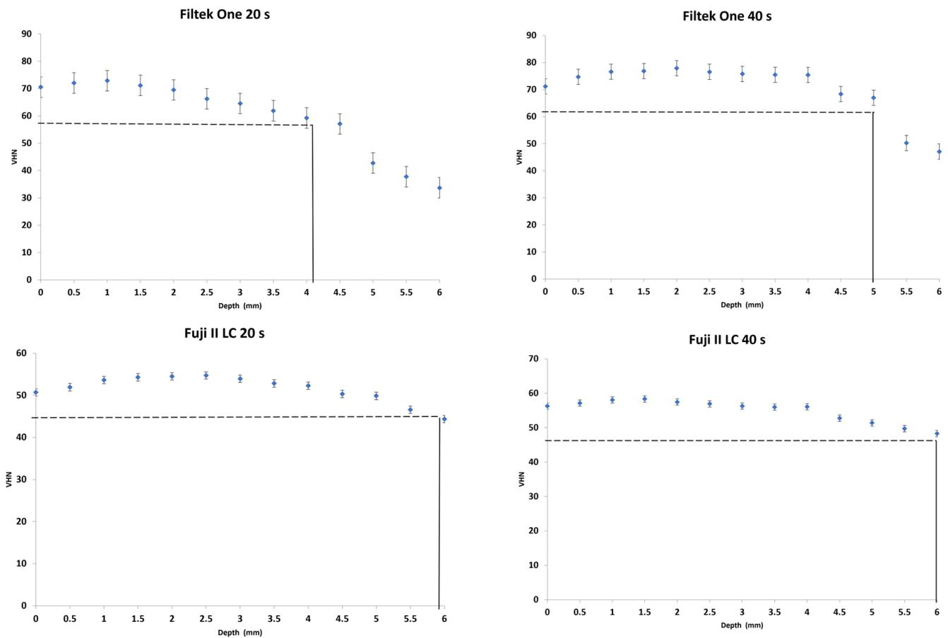
**Figure 2.** VHN at 80% of Max. VHN (dashed line) and depth at 80% of Max. VHN (solid line) of the tested material.
