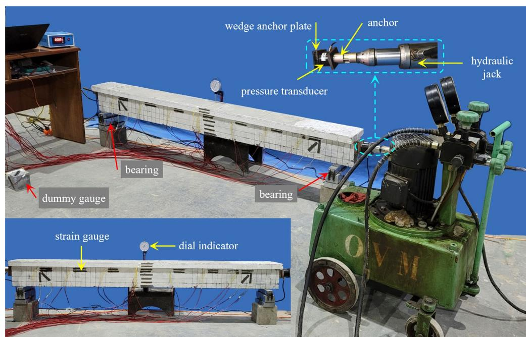
Figure 6. Schematic diagram of prestress tensioning.
