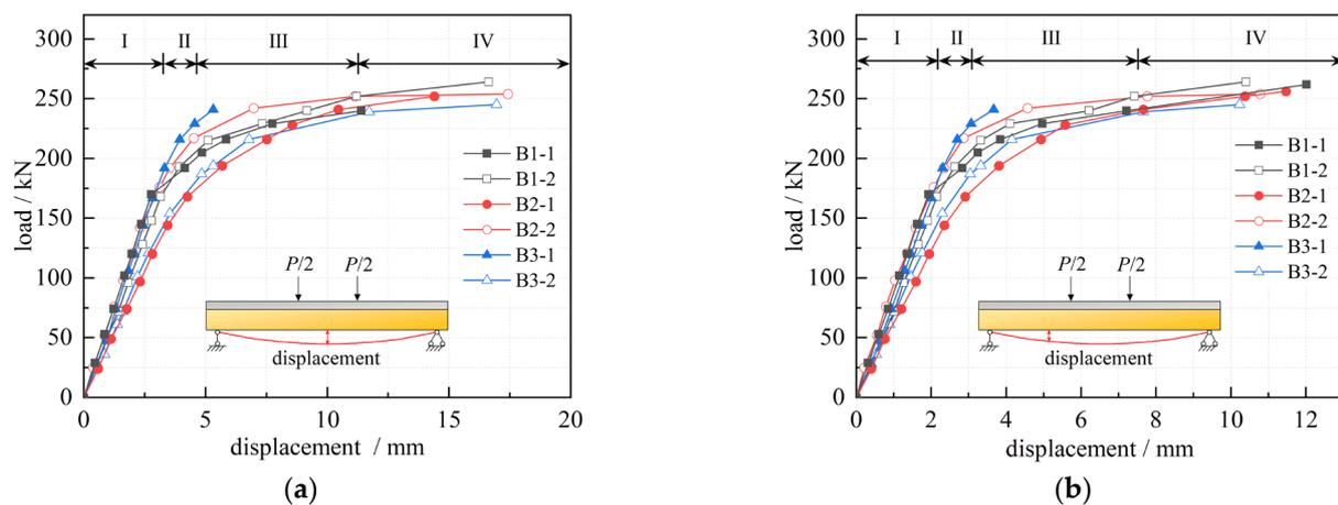
Figure 8. Load-deflection curves; (a) mid-span; (b) 1/4 span.
