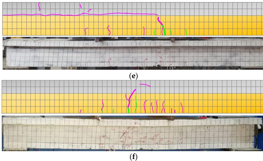
**Figure 10.** Crack distribution results for each beam; (a) B1-1; (b) B1-2; (c) B2-1; (d) B2-2; (e) B3-1; (f) B3-2.
