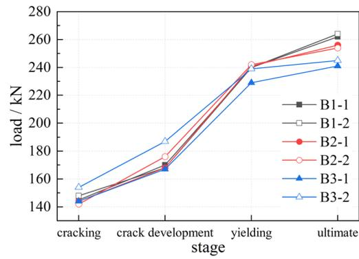
Figure 9. Control load of each stage of beams.
