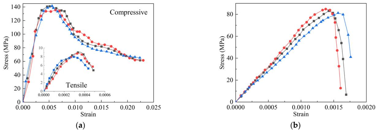
Figure 5. The stress-strain curve; (a) UHPC; (b) NC.
