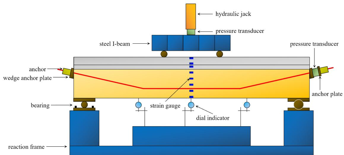
Figure 7. Loading diagram of bending test.
