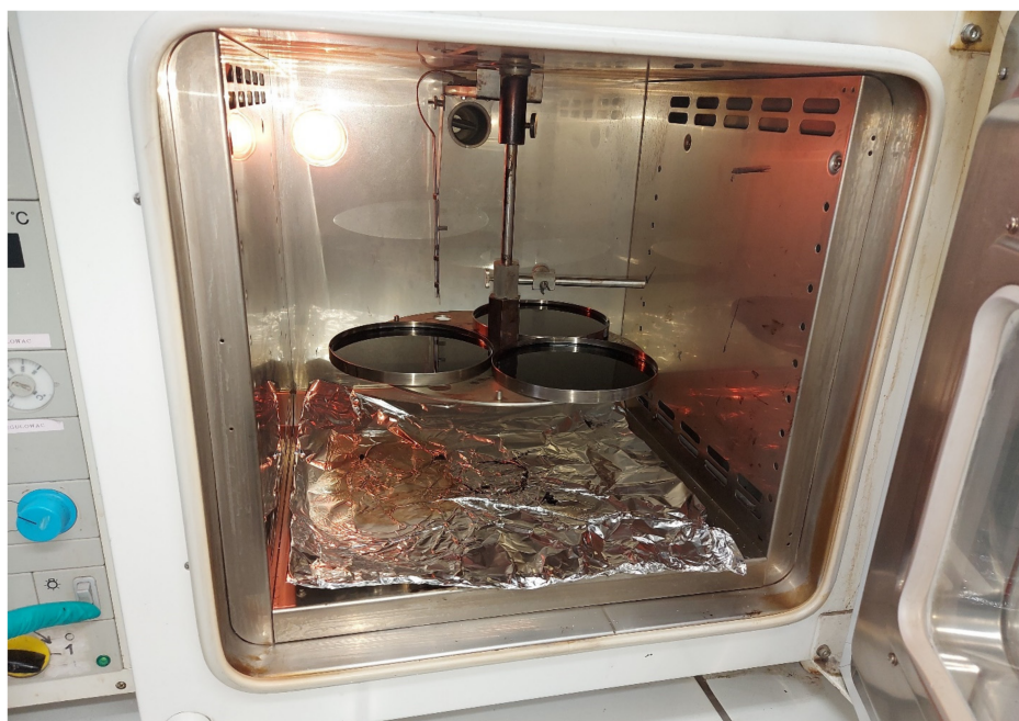
Figure 4. Photograph of a set of pans and an oven for aging bitumen by the TFOT method.
