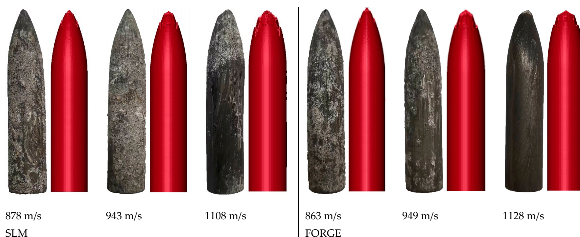
Figure 30. Comparison of projectile wear after penetration at different speeds.
