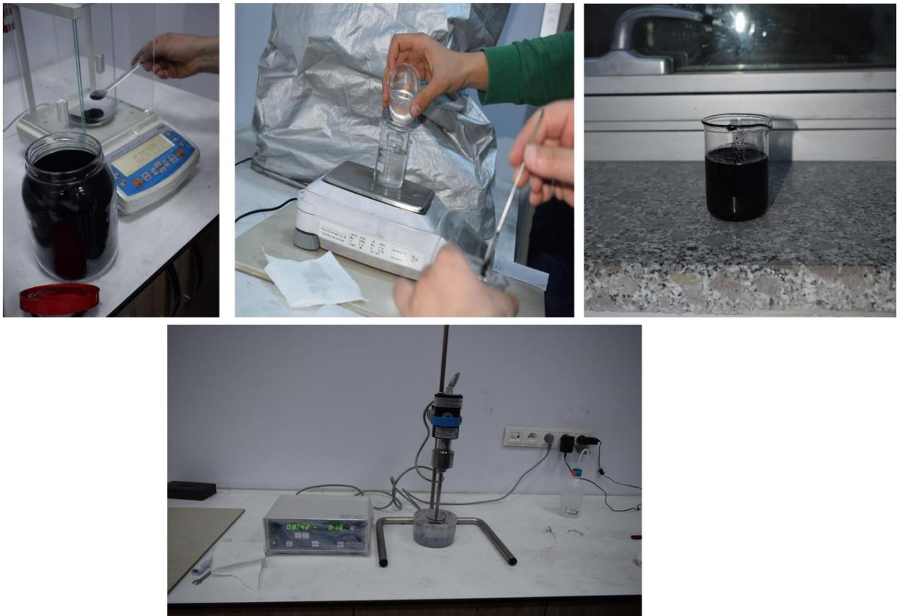
Figure 1. CNTs in epoxy resin and using the mixture of resin/CNT as the matrix of the composite.
