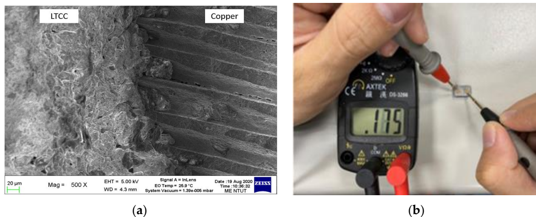
Figure 12. SEM image of the microstructure of the interface between the LTCC ceramic and copper (a) and the electrical conductivity test (b).
