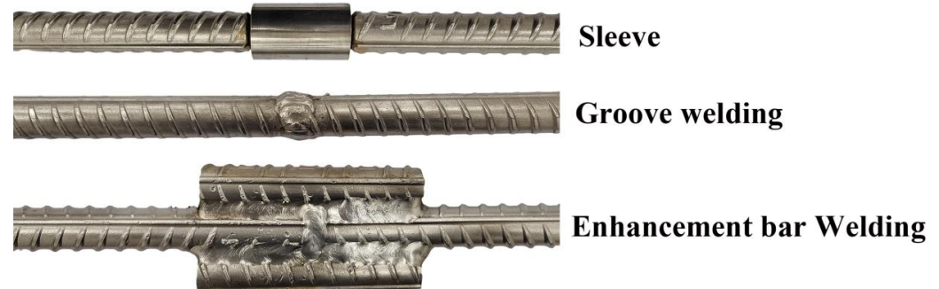
Figure 16. Surface morphology of each joint after rust removal.
