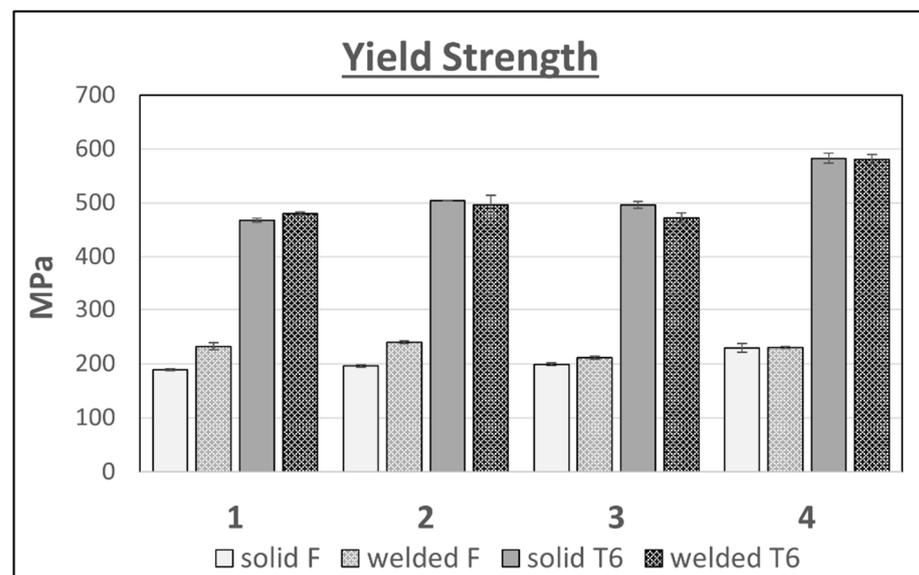
**Figure 9.** Comparison of the yield strength results of flat bars with the weld and solid for 4 variants of alloys in the F and T6 tempers.
