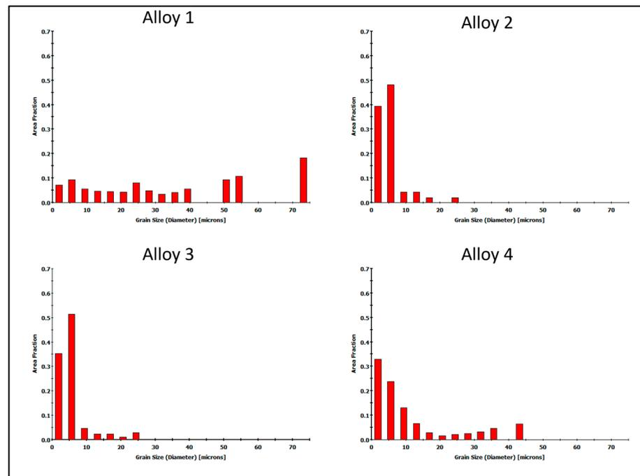
**Figure 13.** Grain size distributions for investigated alloys—welded area of extruded  $60 \times 6$  mm profile. In red—area fraction of specific grain size.
