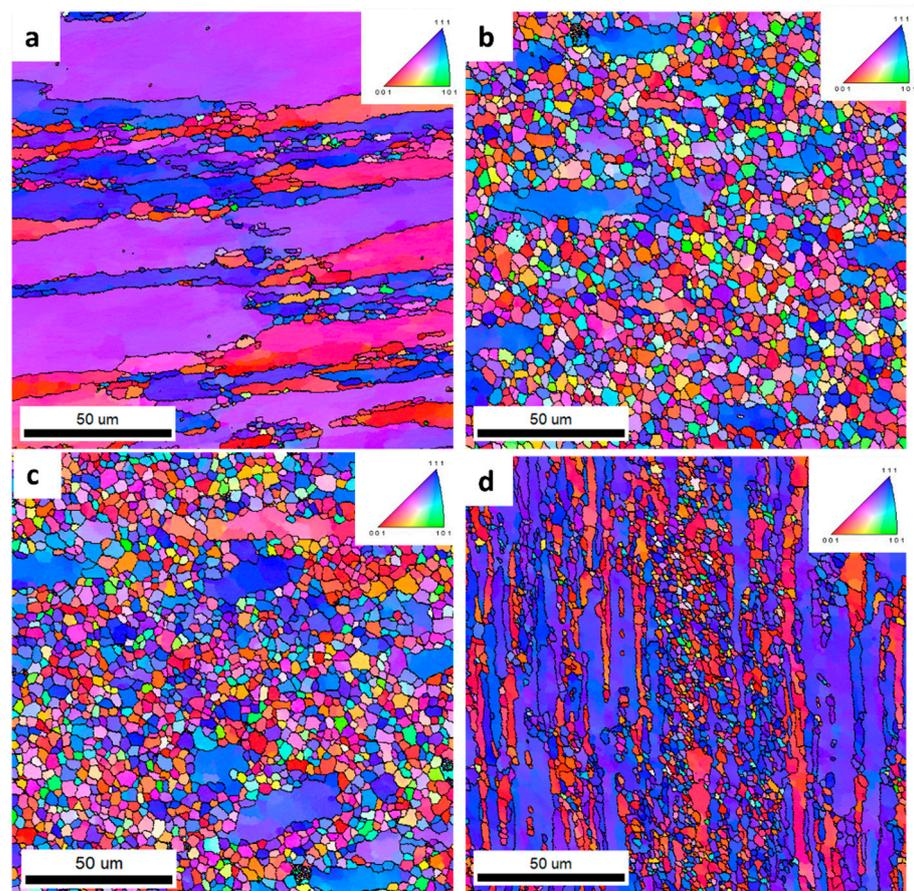
**Figure 12.** IPF images of investigated alloys: 1 (a), 2 (b), 3 (c), and 4 (d)—welded area.
