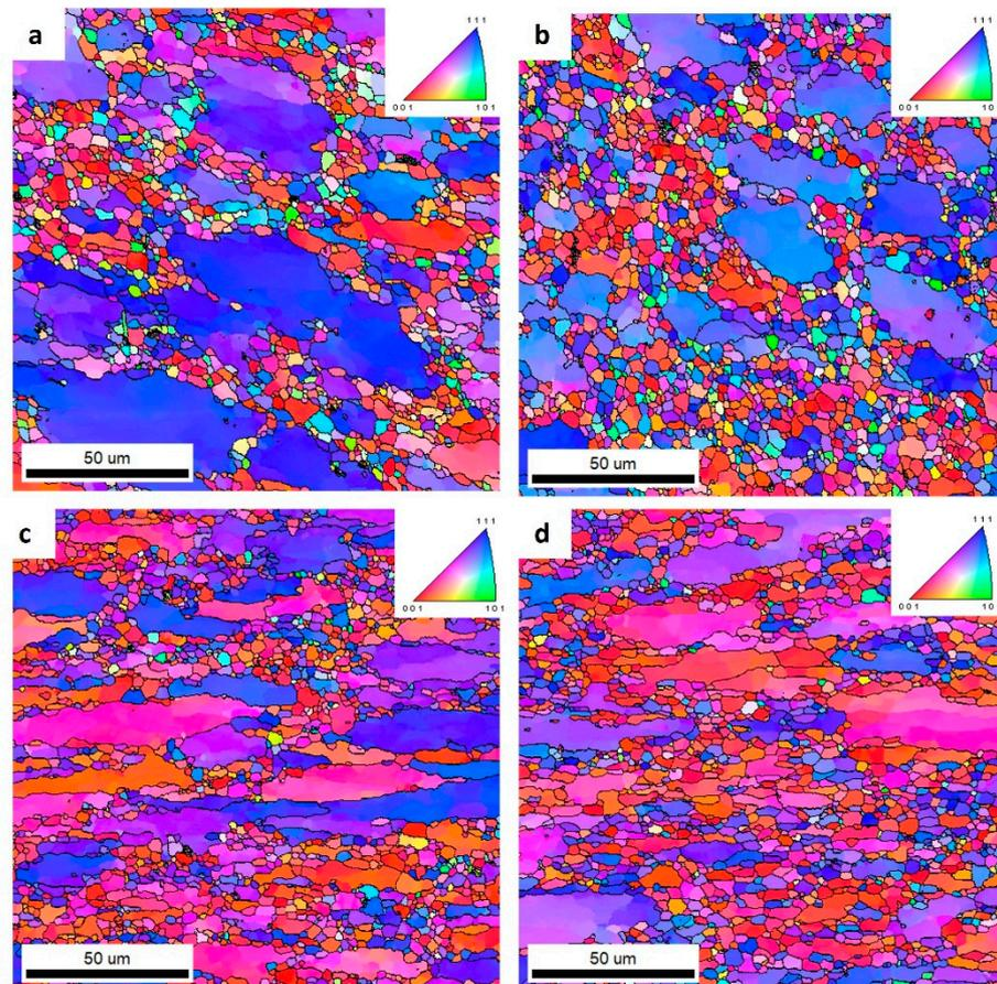
**Figure 14.** IPF images of investigated alloys: 1 (a), 2 (b), 3 (c), and 4 (d)—outside the welded area.
