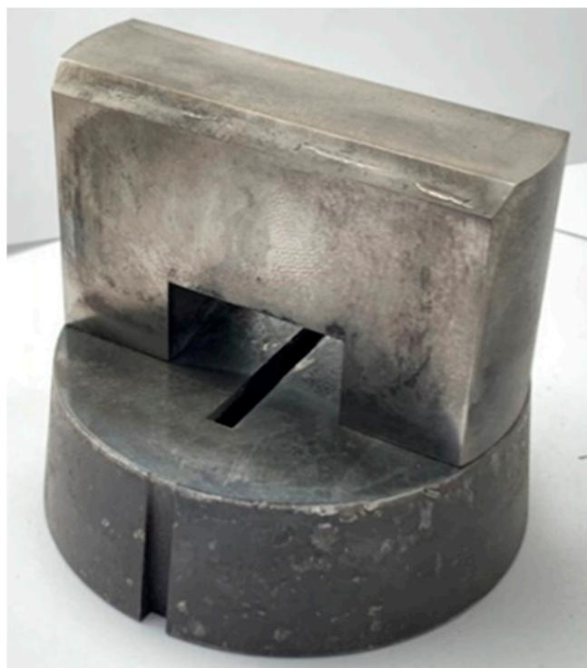
**Figure 2.** A die insert with single bridge used for extrusion of  $60 \times 6$  mm flat bar with weld.
