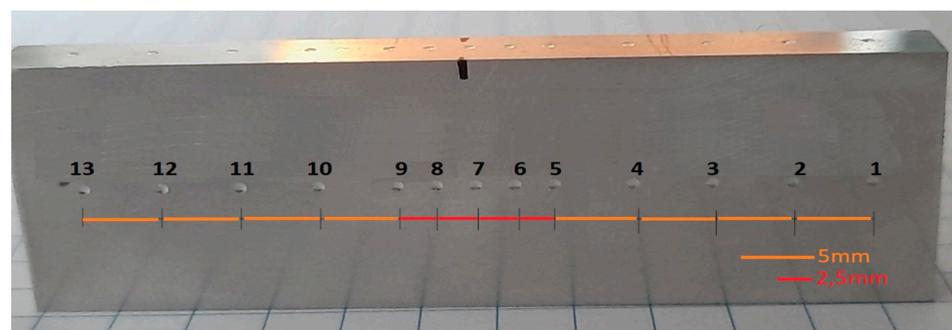
**Figure 5.** An example of the distribution of Brinell hardness test measurement points.
