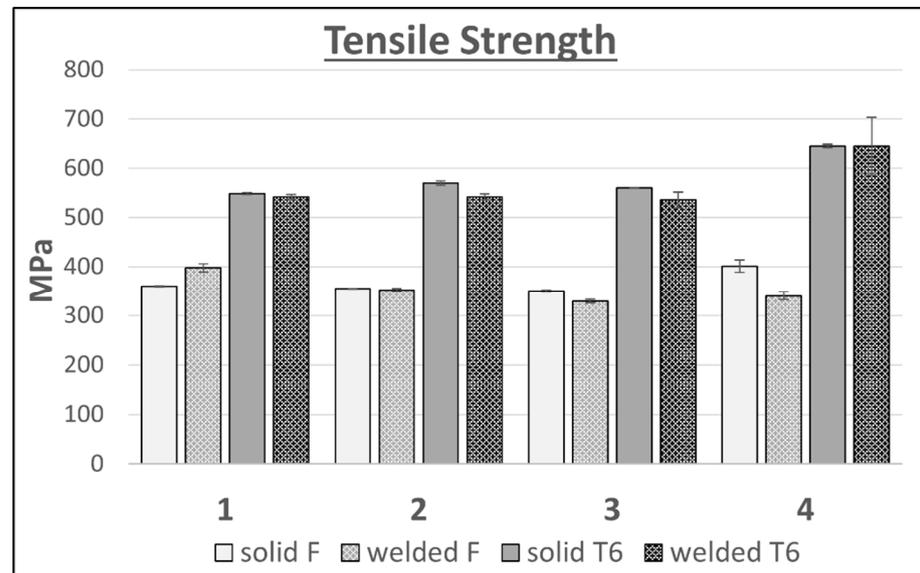
**Figure 8.** Comparison of the tensile strength results of flat bars with the weld and solid for 4 variants of alloys in the F and T6 tempers.
