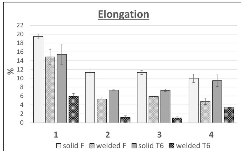
**Figure 10.** Comparison of the elongations of flat bars with the weld and solid for 4 variants of alloys in the F and T6 tempers.
