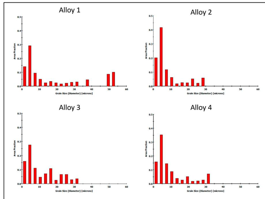
**Figure 15.** Grain size distributions for investigated alloys—outside the welded area of extruded  $60 \times 6$  mm profile. In red—area fraction of specific grain size.
