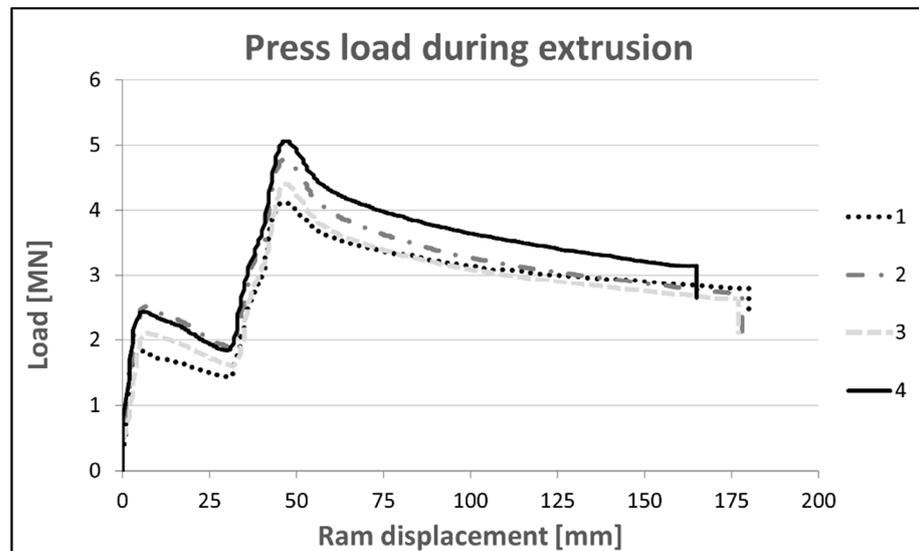
**Figure 6.** Press loads recorded during  $60 \times 6$  mm section extrusion of tested aluminum alloys.
