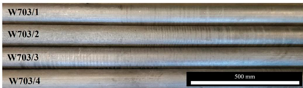
**Figure 1.** Cast billets of the investigated alloys. From the top to the bottom: alloy 1, 2, 3, 4. W703 is the casting batch number.
