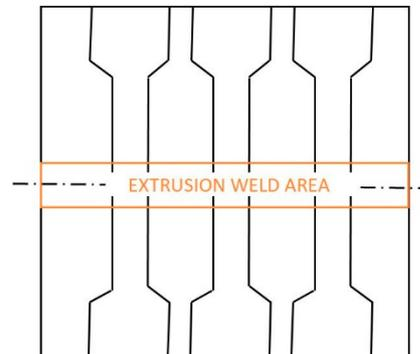
**Figure 4.** An example of sampling for static tensile test.
