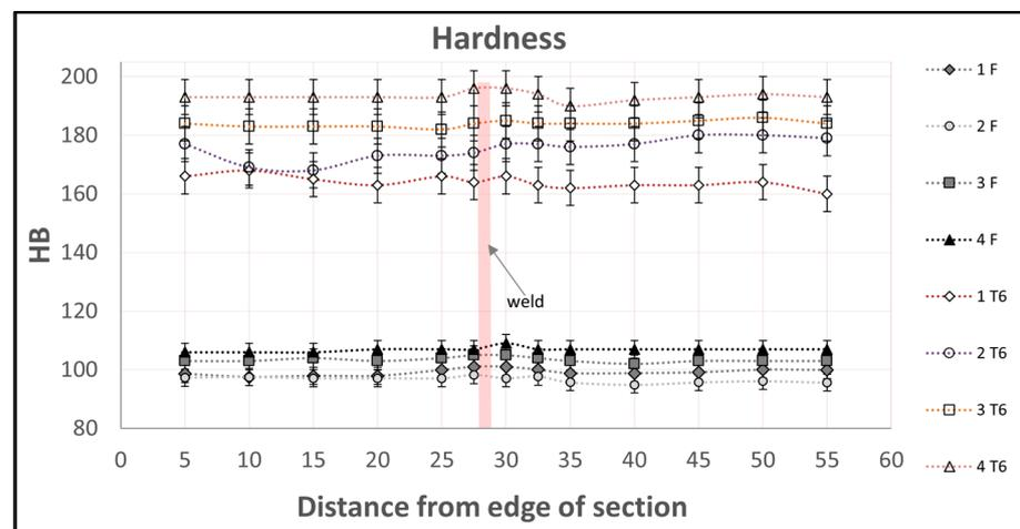
**Figure 7.** Hardness distributions [HB] on cross-sections of the flat bar  $60 \times 6$  mm: at the top—after heat treatment of the T6 temper; at the bottom—in the F temper.
