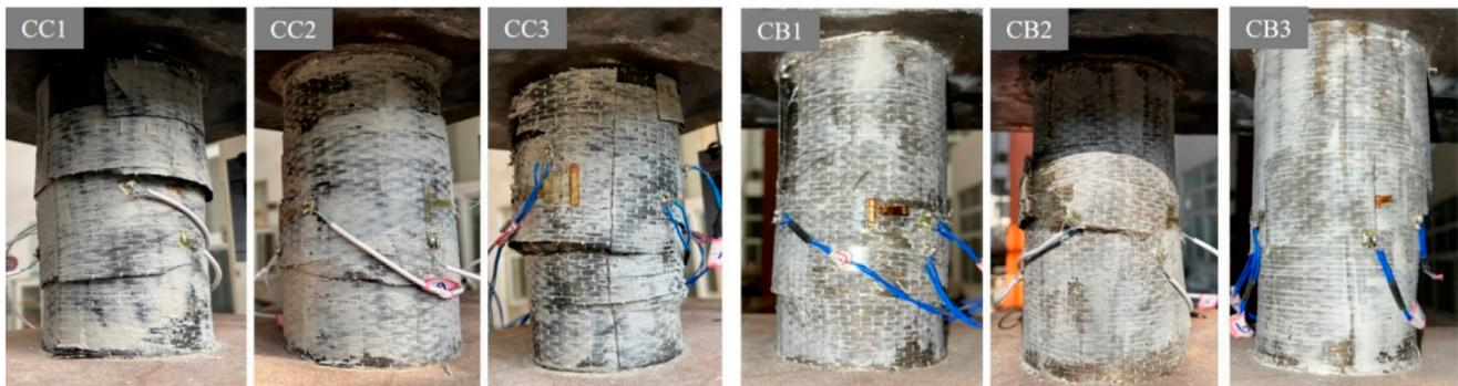
**Figure 6.** Pictures of the composite columns after destruction.
