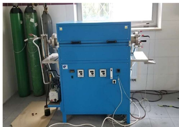
Figure 7. Laboratory pyrolysis furnace for the biochar production system.
