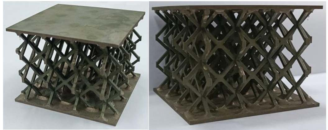
Figure 2. Specimens of the brazed hourglass lattice sandwich structure.
