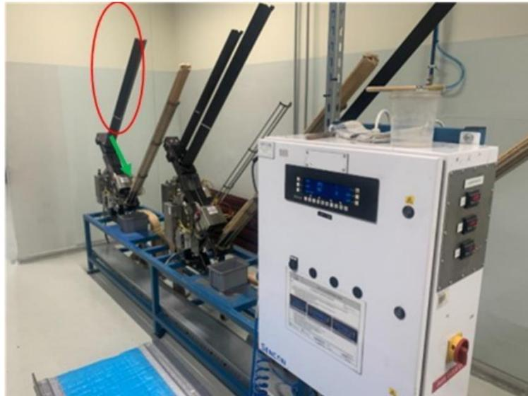
**Figure 7.** Beverage end leak tester.
