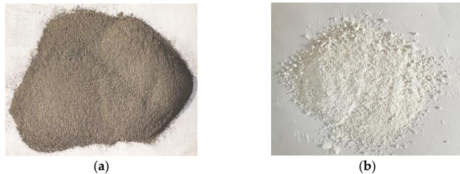
Figure 1. Steel slag powder (a) and metakaolin (b).
