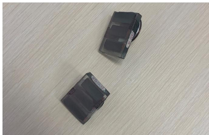
**Figure 5.** Section samples for scanning microscope examination.
