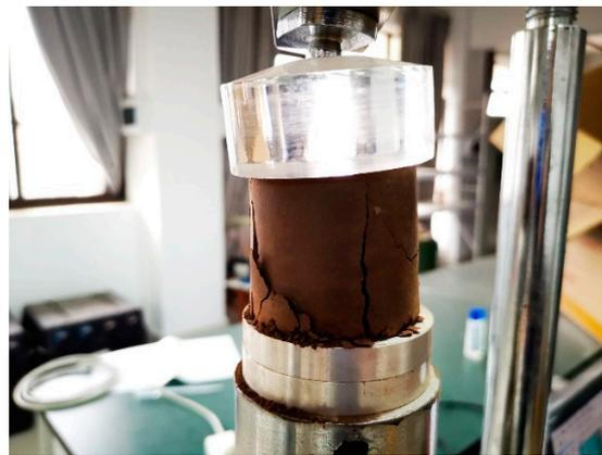
Figure 3. Specimen damage by compression.
