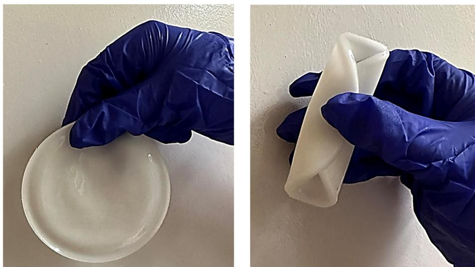
**Figure 1.** Pictures of rose-modified hydrogel materials (sample 50/3).
