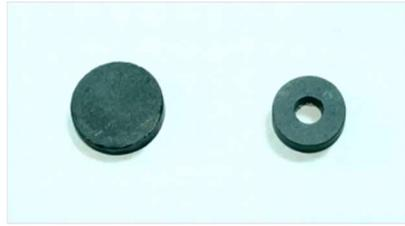
**Figure 1.** The green body of a  $\text{Ba}_{0.6}\text{La}_{0.2}\text{Sr}_{0.2}\text{Co}_2\text{Fe}_{16}\text{O}_{27}$  hexaferrite disc (left) and toroidal specimen (right).
