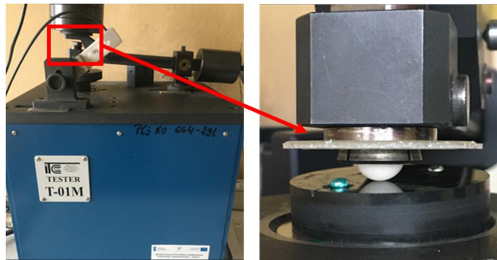
**Figure 2.** T-01 tribological tester and the  $\text{Al}_2\text{O}_3$  ceramic ball-on-disc.
