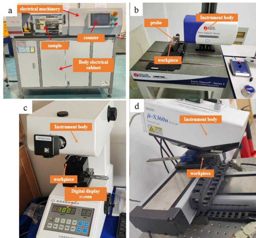
Figure 3. (a) QBWP-1000 cantilever bending fatigue testing machine; (b) New View 5022 surface profiler; (c) automatic microhardness tester; (d)  $\mu$ -X360n X-ray residual stress analyzer.
