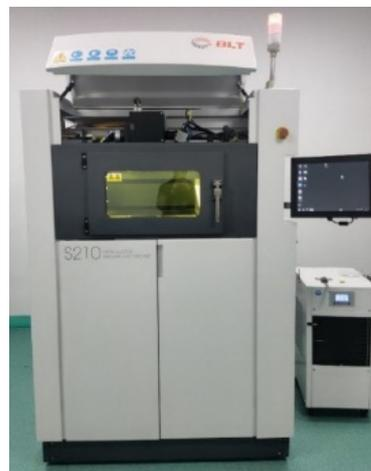
**Figure 6.** BLT-S210 SLM forming equipment.
