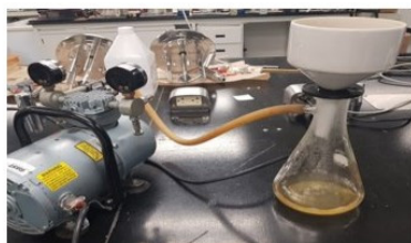
2. Filtration of the mixture and recovery of the filtrate.
