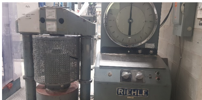
Figure A3. RIEHLE, Baden-Württemberg Germany compression/tension tester.
