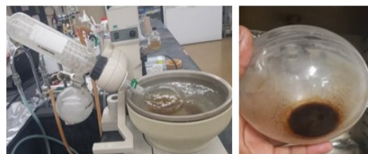
3. Rotavapor extraction: evaporation of distilled water and recovery of hemp fibers/hurds soluble compounds.
