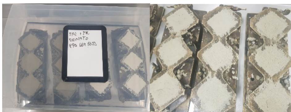
Figure A2. Cement paste preparation for compression tests.
