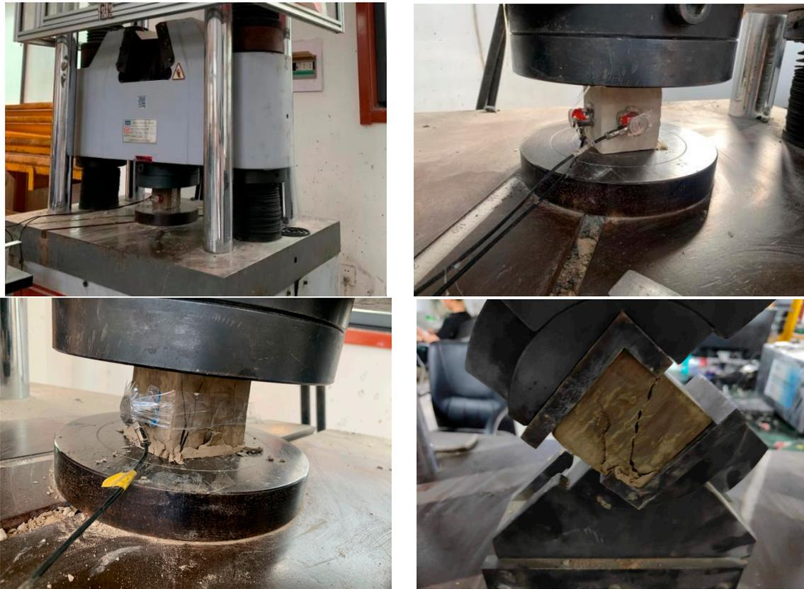
**Figure 5.** Compressive strength test and some details of the failure modes of loaded specimens.
