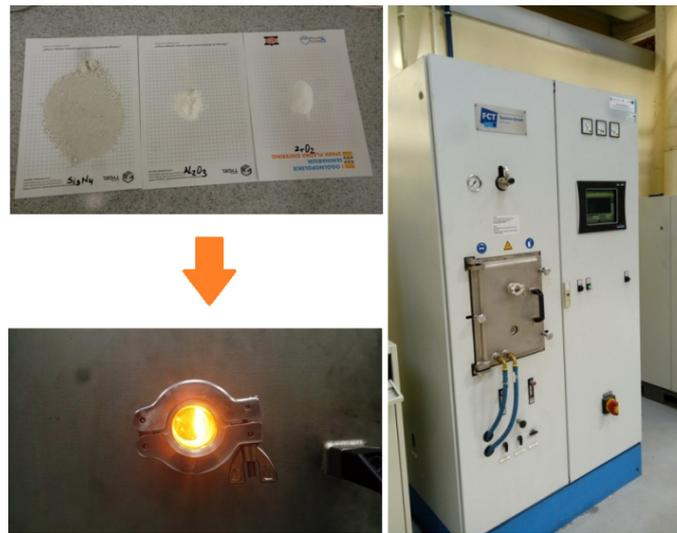
**Figure 3.** View of the spark plasma sintering furnace (FCT Systeme GmbH, Frankenblick, Germany) used to produce the ceramic composite [Proprietary development].
