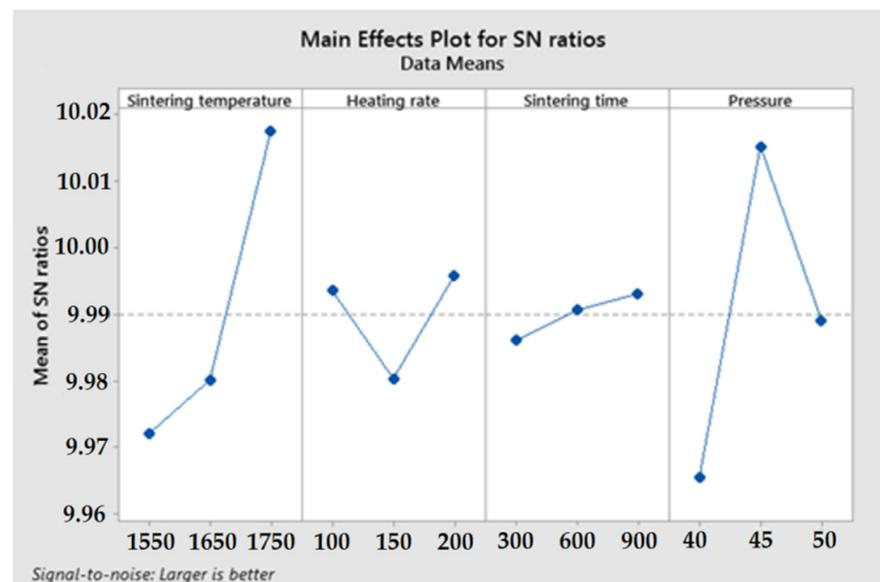
Figure 5. Mean Signal-to-Noise Ratios based on sintering test results.
