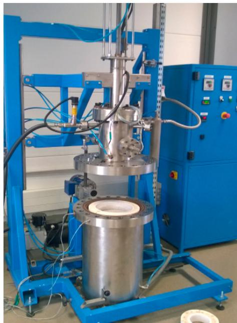
**Figure 1.** A view of a device intended to infiltrate a porous ceramic material under gas pressure.
