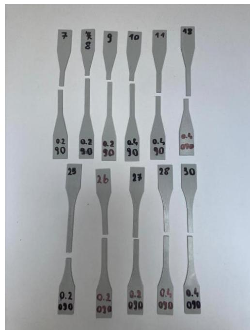
**Figure 5.** Specimens from the 3rd set of measurements with the correct breaking location.
