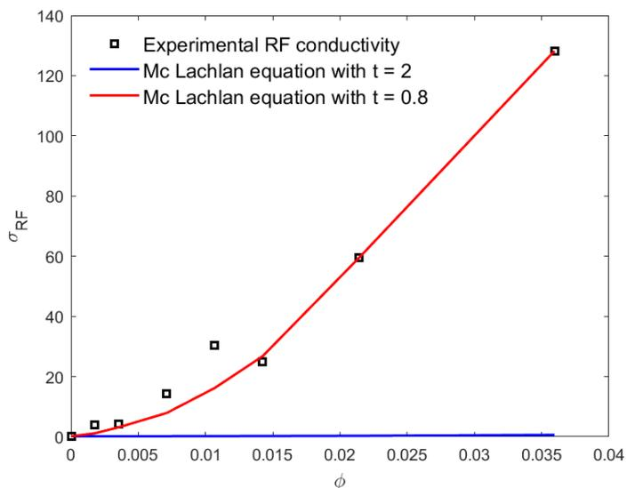
**Figure 6.** RF conductivity as a function of CNT volume fraction. The full squares are the measurement; the solid curve is a calculation based on the McLachlan equation, Equation (2), with  $t = 2$ , and the dash-dotted curve is a calculation based on Equation (10) with  $t = 0.8$ .
