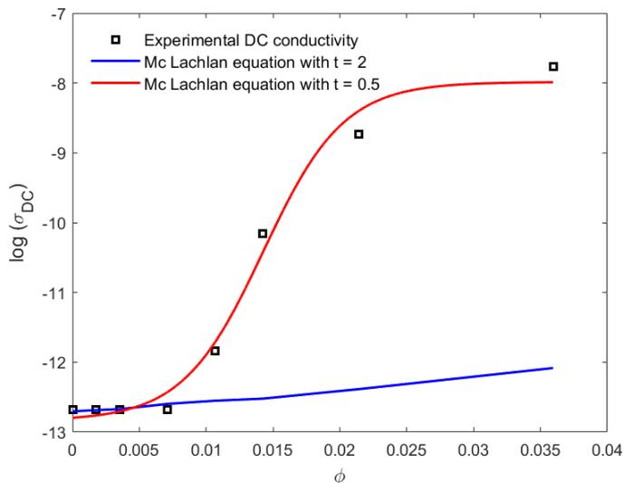
**Figure 5.** DC conductivity as a function of CNT volume fraction. The full squares are the measurement; the solid curve is a calculation based on the McLachlan equation, Equation (2), with  $t = 2$ , and the dash-dotted curve is a calculation based on Equation (10) with  $t = 0.5$ .
