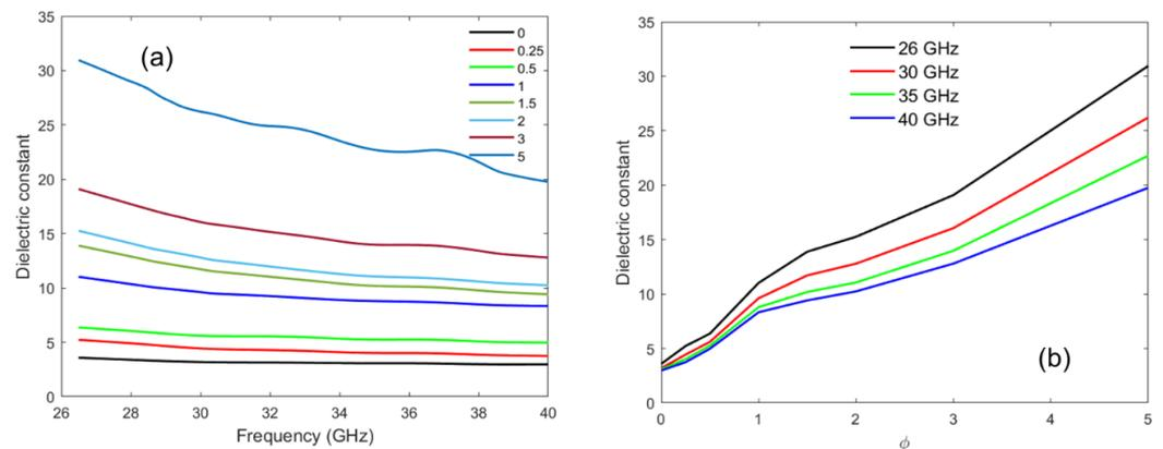
**Figure 7.** Dielectric constant as a function of frequency (a) and CNT weight fraction (b).
