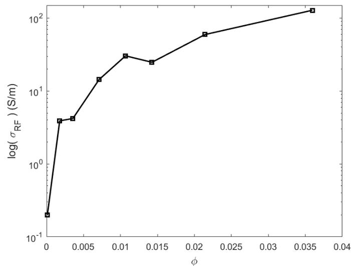
**Figure 2.** Logarithm of the microwave RF conductivity averaged over the Ka frequency range in function of CNT volume fraction.
