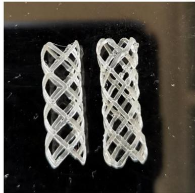
**Figure 15.** Image of the BVS made by the four-axis printing method: as printed (**left**) and after the shape recovery (**right**).
