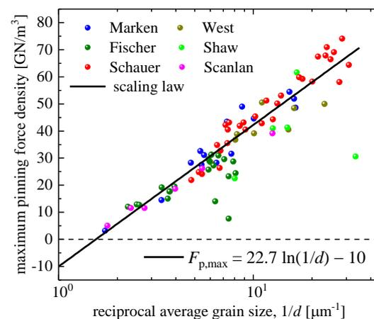
**Figure 2.** Maximum pinning force density,  $F_{p,max}$ , vs. reciprocal average grain size,  $1/d$ , for datasets reported by Marken [46], West et al. [47], Fischer [44], Shaw [48], Schauer et al. [49], and Scanlan et al. [50]. Fitting curve (Equation (3)) was proposed by Godeke [45], who also presented the full dataset in a log-linear plot.
