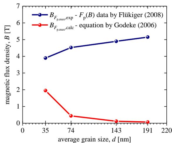
**Figure 3.**  $B_{F_{p,max,calc}}$  was calculated using Equation (4) (red) [45] and  $B_{F_{p,max,exp}}$  was extracted from experimental data reported by Flükiger [41] for Nb<sub>3</sub>Sn conductors fabricated by bronze technology.
