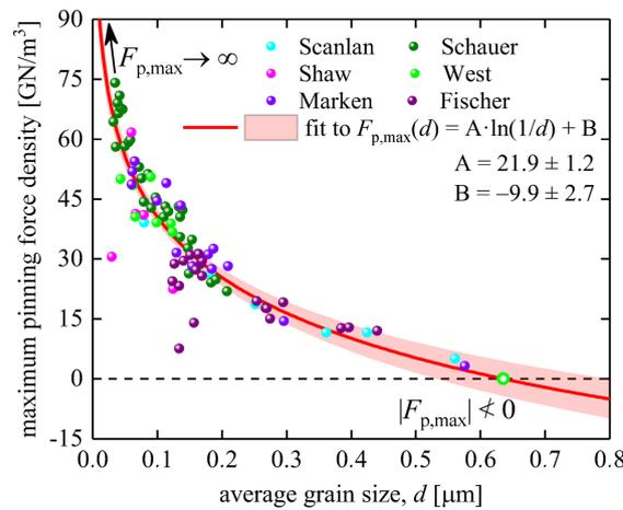
**Figure 4.**  $|F_{p,max}(d)|$  data from Figure 2 (reported by Fischer [44] and Godeke [45]) in a linear–linear plot, and the fitting curve to Equation (3) [45], where we also showed both side extrapolations within the average grain size range of  $20 \text{ nm} \leq d \leq 800 \text{ nm}$  of  $\text{Nb}_3\text{Sn}$ . Raw data reported by Marken [46], West et al. [47], Fischer [44], Shaw [48], Schauer et al. [49], and Scanlan et al. [50]. Pink shaded areas show the 95% confidence bands.
