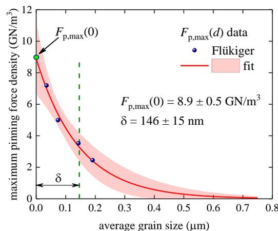
**Figure 7.** Maximum pinning force density,  $|F_{p,max}(d)|$  vs. average grain size,  $d$ , and data fit to Equation (15) for samples fabricated by bronze technology and data fit to Equation (15). Raw data reported by Flükiger et al. [41]. Deduced parameters are  $|F_{p,max}(0)| = 8.9 \pm 0.5 \frac{\text{GN}}{\text{m}^3}$ ,  $\delta = 146 \pm 15 \text{ nm}$ . Fit quality is 0.9837. The pink shaded areas show the 95% confidence bands.
