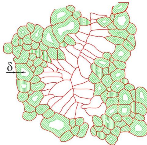
**Figure 8.** Schematic representation of the effective areas ( $\delta$ -layer) in a cross-section of the equiaxed Nb<sub>3</sub>Sn layer.
