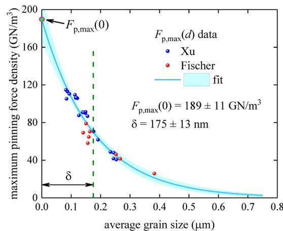
**Figure 6.** Maximum pinning force density,  $|F_{p,max}(d)|$  vs. average grain size,  $d$ , and data fit to Equation (15) for the A15 layer fabricated by powder-in-tube technology [44,60]. Raw data reported by Fischer [44] and Xu et al. [60]. Deduced parameters are  $|F_{p,max}(0)| = 189 \pm 11 \frac{\text{GN}}{\text{m}^3}$ ,  $\delta = 175 \pm 13 \text{ nm}$ ; fit quality is 0.9093. The cyan shaded areas show the 95% confidence bands.
