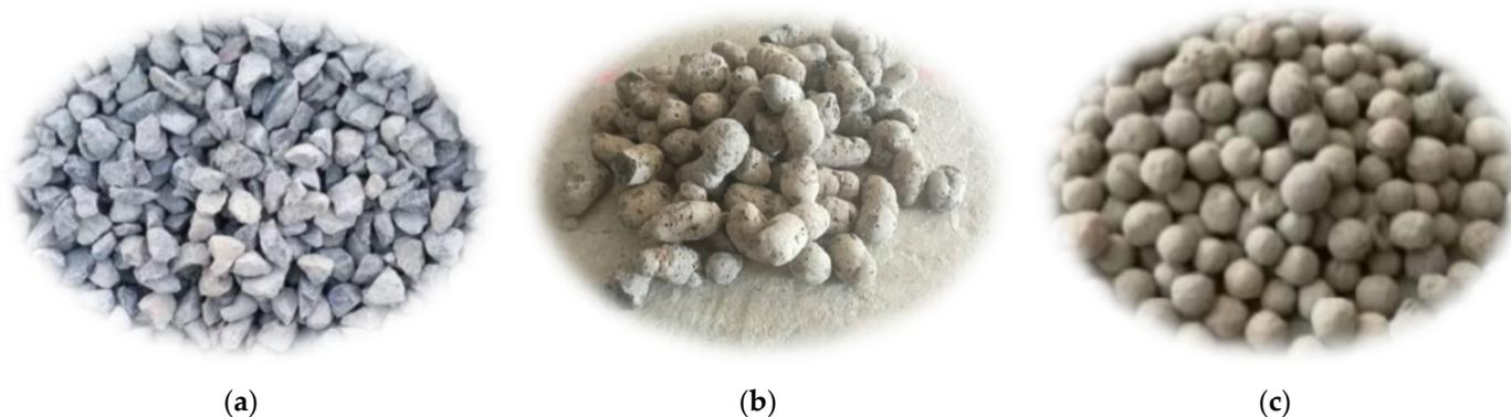
**Figure 1.** The aggregates used in this study: (a) ordinary crushed-stone aggregates; (b) lightweight ceramsite; (c) high-strength clay ceramsite.
