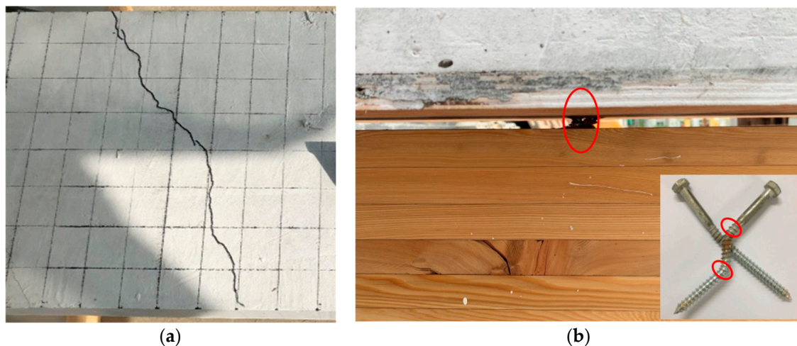
Figure 3. Push-out test phenomenon. (a) Cracks of concrete slab; (b) Pulling out failure of screw fasteners.
