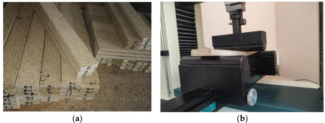
**Figure 2.** Determination of bending strength: (a) preparation of specimens for bending strength tests; (b) specimen during testing between press supports.
