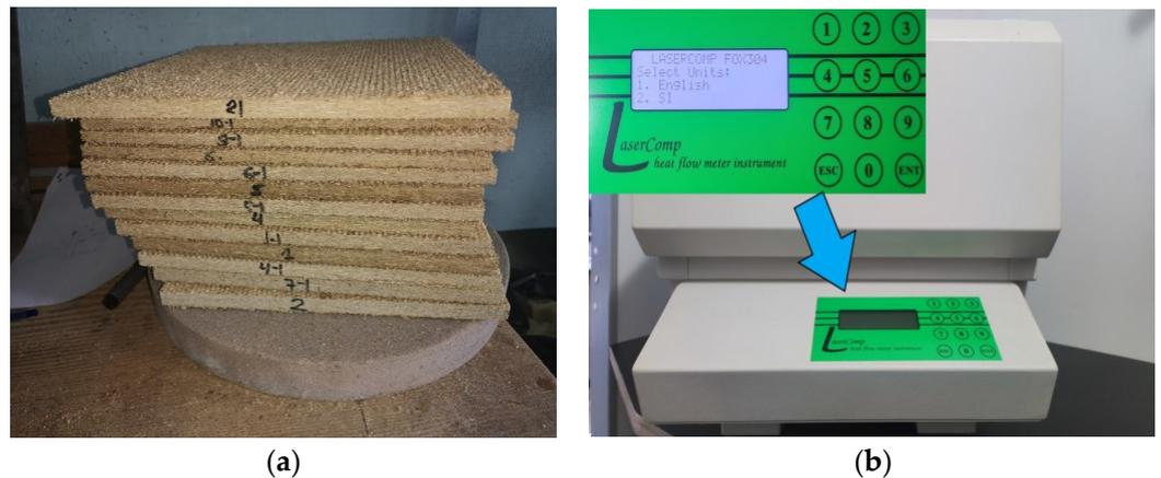
**Figure 3.** Thermal conductivity studies: (a) preparation of specimens; (b) determination of the thermal conductivity coefficient of the specimens in the FOX 304 device.
