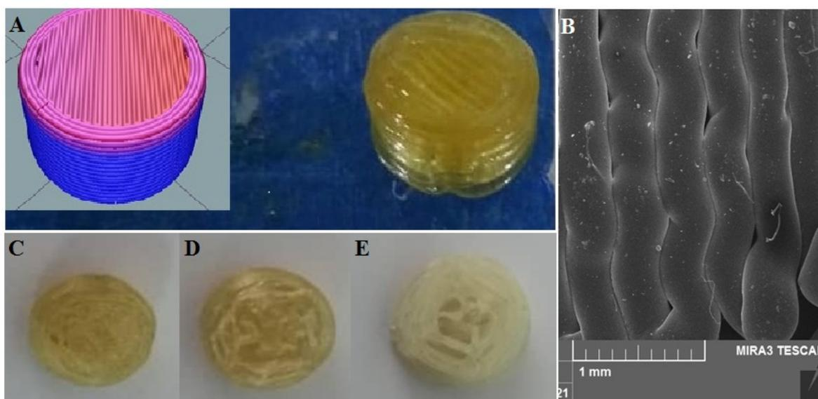
**Figure 1.** Representative images of 3D-printed pill of tacrolimus (A), inset shows the sliced version by software; SEM micrographs of printed layers of PVA filaments (B); cross-section of 3D-printed pill with (C) 90% infill; (D) 50% infill; and (E) 10% infill.
