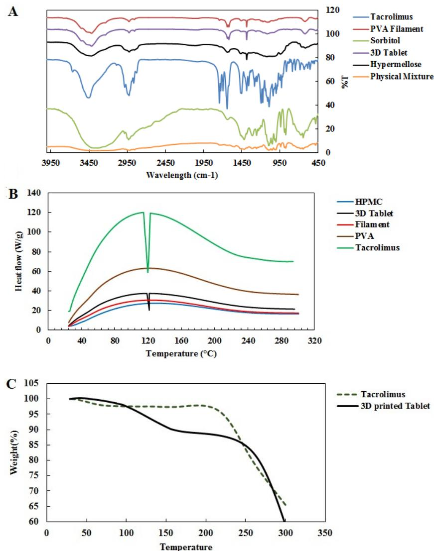
**Figure 2.** FTIR spectrum of 3D-printed pills (A); DSC thermogram of 3D-printed tacrolimus pills and their ingredients (B); thermogravimetric analysis of tacrolimus monohydrate and 3D-printed tablet (C).
