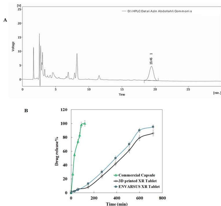
**Figure 3.** Representative HPLC chromatogram of injected samples of assay solution (A); dissolution profile of 3D-printed tacrolimus of 5 mg in comparison with “ENVARSUS” XR tablet and commercial tacrolimus capsule (B).
