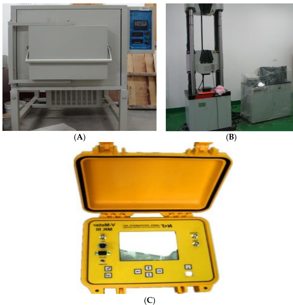
Figure 4. Test equipment. (A) SMF1900-50 Chamber Resistance Furnace. (B) Rigid Servo Triaxial Compression Tester. (C) 2V-METER III Ultrasonic Pulse Velocity Tester.
