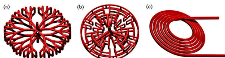
**Figure 38.** Fractal-tree-like heat sink designs: (a) Y-type; (b) H-type; and (c) traditional helical tube [216].
