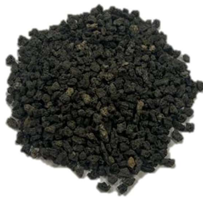
Figure 1. Pumice lightweight fine aggregate.
