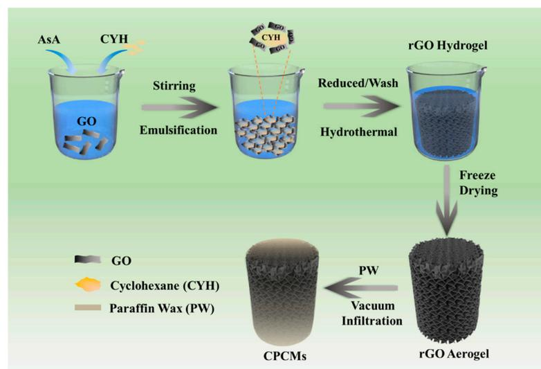
**Figure 1.** A schematic description of the preparation of the three-dimensional rGO-aerogel-based phase-change materials.
