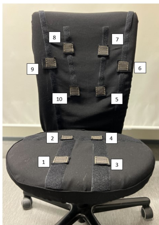
Figure 1. Smart chair with sensor distribution and number identification.
