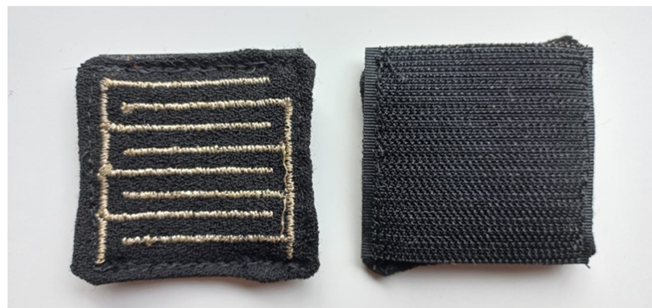
Figure 4. Ready-made sensor from both sides.
