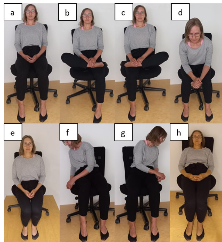
Figure 6. Measured sitting positions during the smart chair test. (a). Ergonomic posture, (b). Right leg crossed, (c). Left leg crossed, (d). Detach from the backrest, (e). Sit on the edge, (f). Lean to the right, (g). Lean to the left and (h). Lean back and sit on the edge.
