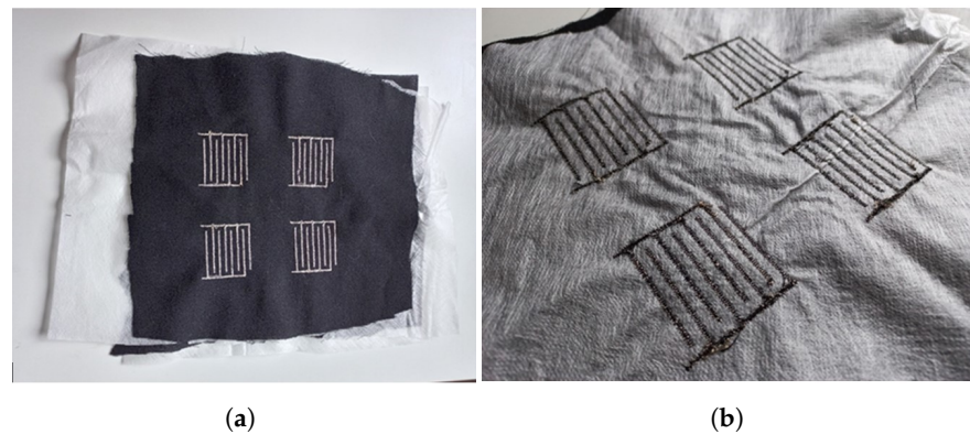
Figure 3. PreCaTex sensor embroidered with the Husqvarna Viking Designer Ruby Royale. (a) Top side of the sensor. (b) Bottom side of the sensor.
